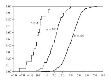
EDFs for three samples of sizes 20, 100, and 500 drawn from three normal distributions, each with variance 1 and with means 0, 2, and 4, respectively
